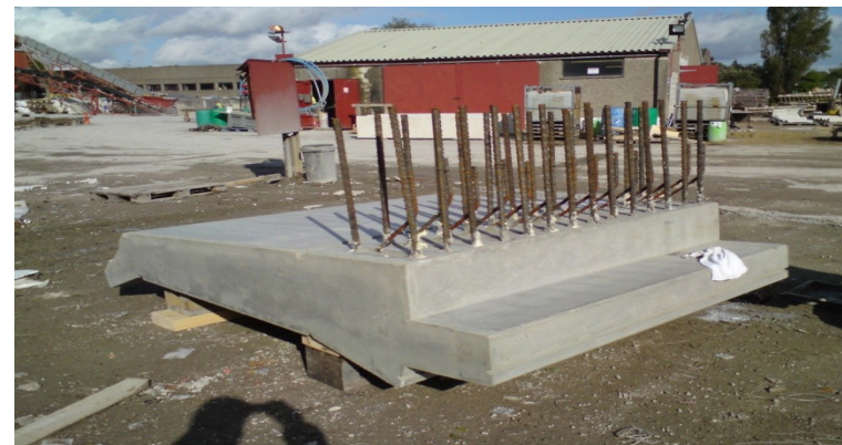
This concrete parapet is from the mould pictured far left. This mould was manufactured for Evans Concrete & was for part of an Olympic project.
