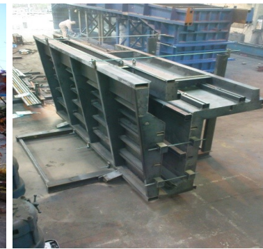
All parapet moulds have internal ends so different width units can be cast.
