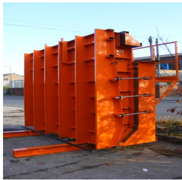
Evans Concrete – H4A Parapet.
