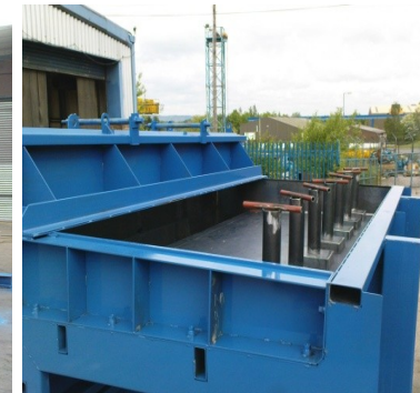
Removable cores which the client chose to remove whilst the concrete was “green”.
